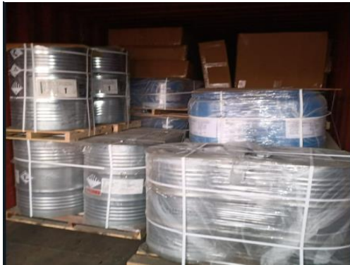
Drums not corrected lashed to container
