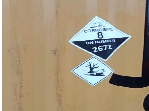
Incorrect exterior container Placarding
