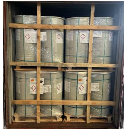
Load correctly loaded
