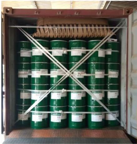
Correct Drum type, lashing to prevent movement
