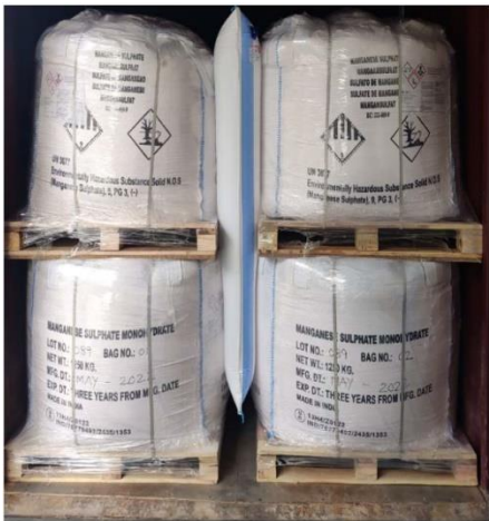
Airbags used to prevent movement during shipping
