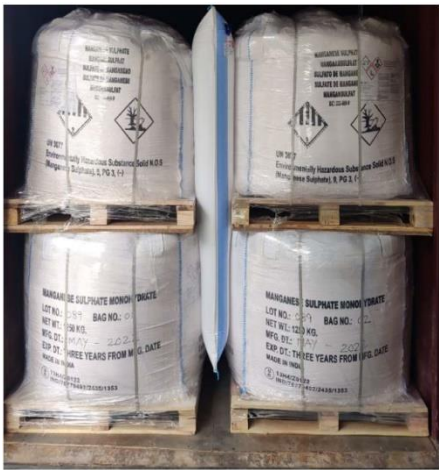
Airbags used to prevent movement during shipping
